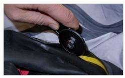
**1.5** Push the Neck Tite Tool forward along the Lock Ring until all of it has been forced into the groove in the Neck Ring. (Strive to get the same amount of excess part of seal around the entire assembly, see image **1.6.**)
