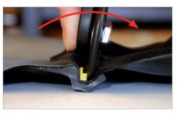
**2.3** When the tool has reached the bottom of **2.4** Press up the Lock Ring from the groove. the groove, it's time to use the tool to bend up the Lock Ring from the groove.
