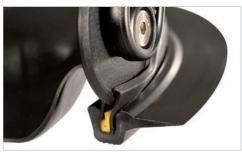
**1.3-1.4** Put the Neck Tite Tool in position as image displays. By applying force, press the Lock Ring down into the tapered groove of the Neck Ring so that the Lock Ring enters the groove and locks into position. **Use a flat surface when performing this operation.**
