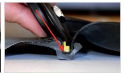
2.2 Press the tool in the direction of the arrow and force the groove in the Neck Ring to "open up" and start releasing the Lock Ring.
