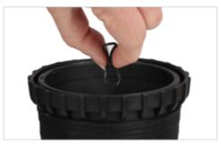
**1.1** Three O-rings should be installed into each **1.2** Pinch the O-ring and insert it from the top
