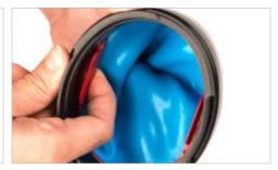
4. Stretch the seal from the inside of the drysuit and at the same time press the ANTARES Support Ring to its final position. No part of the seal shall then be visible between the ANTARES Support Ring and the ANTARES Oval Stiff Ring.
