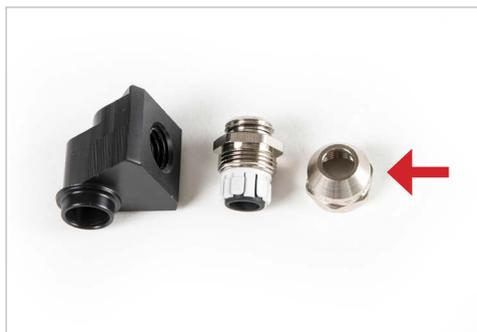
**2.1** Dismantle the cable entry swivel down to three components as shown in this picture. The arrow explains the path of the cable when installing it. Assembling of the swivel components shall be made after the cable has been installed and measured according to preferred length.
