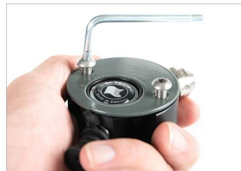
**1.1** Loosen and remove the screws on the cover lid using the 4 mm Allen key. Remove the lid. Make sure to hold the valve upright to prevent components from falling out.
