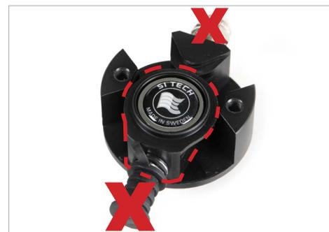
**1.3** The next step is to remove the swiveling components. Start with the inflation assembly. Do not remove it by grabbing the inflation nozzle marked by "X"! Grab the piece within the dashed line area and lift it straight up. Ensure that the O-ring on the valve neck is still in position. The next step is to remove the cable side swivel. Use the same procedure for the removal.
