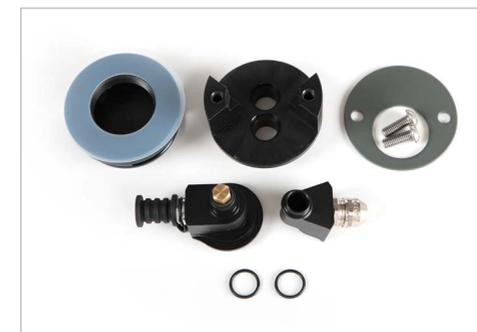
**1.4** These are the components that you have disassembled to this point. Ensure that the O-rings are undamaged and that the O-ring grooves are clean.
