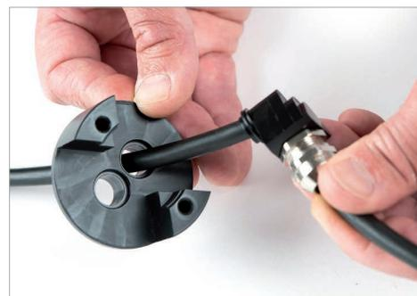
**2.7** Mount the swivel into the valve body, make sure that the O-ring is undamaged and in place. It does not matter which entry you use as the construction of the valve allows both.
