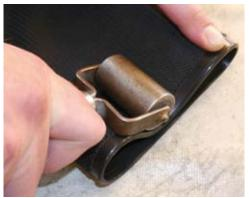
When the adhesive has melted and the ring is in place you need to squeeze away all air-pockets in order to get maximum grip between the components. Use a roller or similar tool to put equal force over the actual surface. Roll back and forth until you have covered the complete surface 360°. When this is done we recommend you to wait about 10 minutes before starting the next step.
