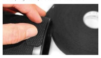
Pre-cut the tape for a rounded edge.
