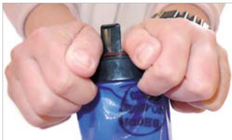
4.5 Press the glove and Oval Spanner Ring so that it bottoms in the Oval Glove Ring. Perform this procedure 360° around the ring.
