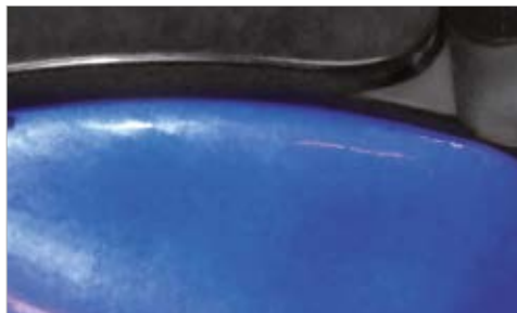
4.4 Check for creases on the glove continuously when pressing the Glove/Oval Spanner Ring into final position. The glove should be positioned as displayed in this image.
