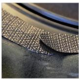
Pre-cut the tape for a rounded edge. Apply two layers of glue on the surface of the ring and the suit (let dry thoroughly in between). To activate; heat the tape and glue on sleeve and ring, 5 cm (2") at a time and stretch the tape gently when applying. When the tape is finally attached you will need to end the attachment with an overlap of approximately 1-2 cm (rounded edges). Use a roller to squeeze out all air bubbles.
