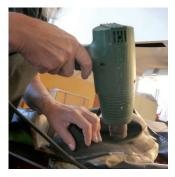
Heat both the Quick Neck Ring and the suit. Move the nozzle of the heat gun constantly to prevent the ring and suit from overheating. Work in areas of 5-10 cm at a time to keep the temperature of the glue at a smooth and constant melting point.
