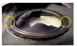
When the last coat of adhesive has dried, it is time to apply the Quick Neck Ring to the drysuit. It is wise to adhere the Quick Neck Ring in the front and back end according to the markings and knobs. When you have fitted the Quick Neck Ring to its actual position you will need to melt the
