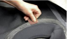
Ensure all surfaces are free from adhesive residues, debris and dirt. This is paramount for the glue to do the job. No matter the adhesive, tools or technique if not cleaned properly, the job will be sub-standard. Roughen the surface with fine emery cloth or sandpaper. Inhouse we use either a table grinder or emery cloth for roughing surfaces. The Quick Neck Ring shall be cleaned and de-greased by the use of acetone for maximum grip properties.
