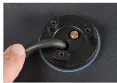
4.3 Mount the valve into the drysuit and 4.4 Bend the cable in preferred direction
