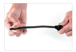
**2.5** Before next step it is important to measure the length of the cable for your specific need. When the nipple is mounted and fastened it will not be possible to adjust the cable in any direction without disassembly.
