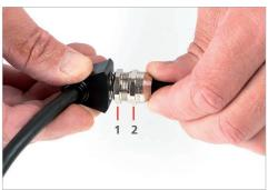
2.6 Mount the nipple into the socket by gently rotating it clockwise, be careful not to damage the thread. Tighten the nipple in two steps:
