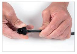
socket is to rotate the cable while pressing it forward into the socket. You may simplify this procedure by using a tool with soft edges! Do not use sharp tools as knifes or similar as you may damage the socket or the cable.
