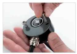
3.3 Put the cover lid in position. Use you fingers to mount the screws and rotate them as far as you can by the force of your fingers. The Allen key must only be used when tightening the screws. Use gentle force when tightening the screws.
