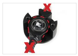
**1.3** The next step is to remove the swiveling **1.4** These are the components that you have components. Start with the inflation assembly. Do not remove it by grabbing the inflation nozzle marked by "X"! Grab the piece within the dashed line area and lift it straight up. Ensure that the O-ring on the valve neck is still in position. The next step is to remove the cable side swivle. Use the same procedure for the removal.
