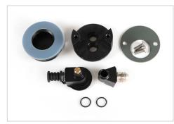
dissasembled to this point. Ensure that the O-rings are undamaged and that the O-ring grooves are clean.
