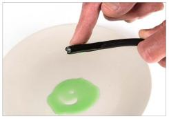
similar product. This will ease up the process of getting the cable through the cable entry components. Ensure that the cable is disconnected from eventual power sources.
