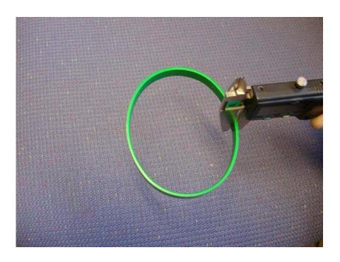
Note that the Spanner ring should be measured at the long side.
