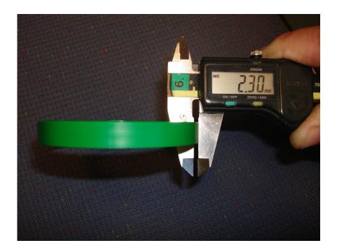
The Spanner ring should be measured with calipers in the middle of the leg.
