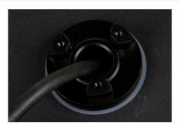
**2.3** Mount the Cable Entry Port into the drysuit and attach the body of the bottom lid. Position the Cable Entry Port in preferred direction and tigthen it by force of hand. Tightening shall be made through rotation of the bottom lid body.
