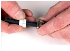
**1.3** Thread the cable through the nipple components as shown in this picture.
