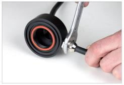
**1.5** Mount the cable and nipple into the Cable Entry Port body. Use a metric wrench (size 18) to gently rotate clockwise. Be careful not to damage the threads.
