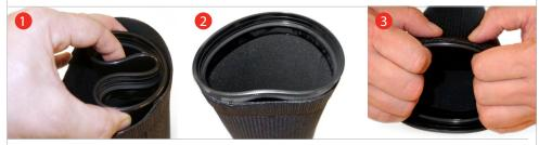
1. Folding the ring will ease the mounting process. 2. Raise the ring and place it with its flange approx. 8-10 mm from the edge of the drysuit arm. 3. Stretch the ring so that it connects to the suit 360°.
