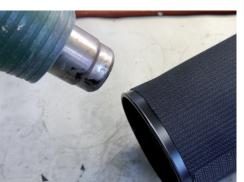
Start by heating the inside of the ring. Move the nozzle of the heat gun constantly, as displayed by the red arrows, to prevent the ring and suit from overheating. The next step is to heat the outside of the drysuit in order to get a smooth and constant melting point of the adhesive.
