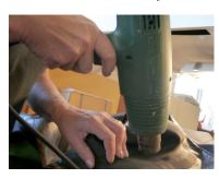
When the second coat of adhesive has dried, it is time to apply the rings to the drysuit. When you have fitted each ring to its actual position you will need to melt the glue by using the heat gun. You must be very careful when using the heat gun. If the fabric of the suit and/or component gets overheated you might damage it.
